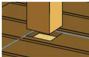
Image C: Tracing a piece of 4x4 on the decking will guarantee an accurate hole.
